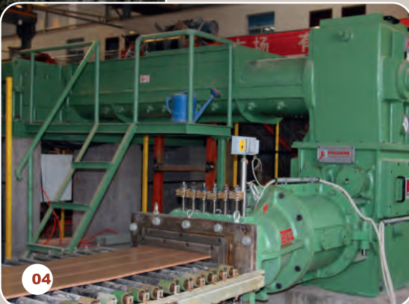
04 Imported Molding Machines of Vacuum Extrusions
