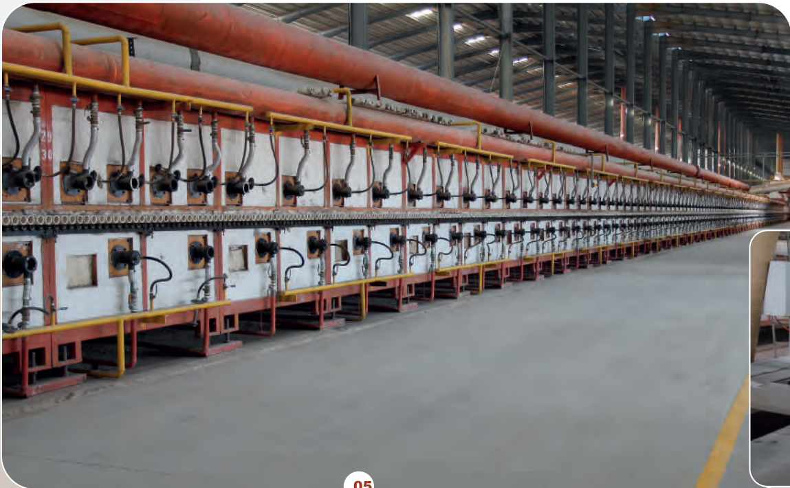
05 Firing Kiln (260 meters, 480 firing units)
