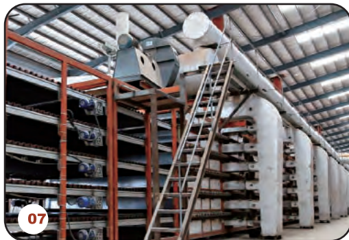
07 Drying Kiln (80 meters, 5 layers)
