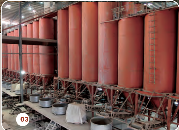
03 Automatic Batching System (115 storage tanks) with Total Material Reserves of 7,000 Tons
